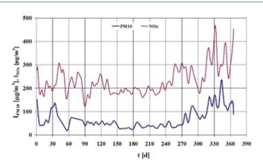
Fig. 1. Immissions of particulate matter PM10 and nitrogen oxides at the air quality monitoring station in Al. Krasińskiego (Cracow)
