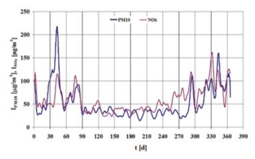
Fig. 2. Immissions of particulate matter PM10 and nitrogen oxides at the air quality monitoring station in Nowa Huta
