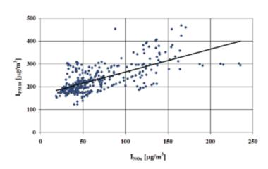
Fig. 5. Correlation dependence of the immission of particulate matter PM10 on the immission of nitrogen oxides at the air quality monitoring station in Al. Krasińskiego (Cracow)
